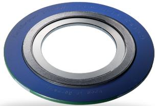
Spiraltherm Graphite S 9584 is a flange seal made from a V-shaped profiled stainless steel tape with spiral-wound graphite middle layer (purity >98 %)
