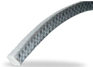
Buraflon 5846 is a diagonally braided, silicone oil-free ramie fiber packing with a light-colored special PTFE impregnating agent based on paraffin wax and oil
